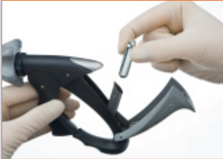
Step 2 Insert CO 2 cylinder
